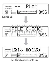
Playback starts automatically from the first file of the first directory once file check is completed. Then, the display changes to show the following:
